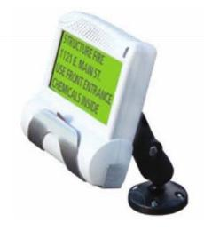
mobile data receiver. The vehicle mount is designed for mounting to your vehicles dashboard, roof, or floor. The custom design allows for permanent mounting or for a "clip & go" feature that allows you to easily remove the RAVENAlert<sup>TM</sup> and take it with you. The vehicle mount uses a custom stainless steel clip attached to an industry standard articulating Ram mounting arm. This allows for total flexibility in locating the device for easy viewing.
