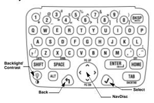
The PageWriter 2000X Two-Way Wireless Communications Center comes with a QWERTY keyboard. Special control keys and key combinations provide the following functions.
