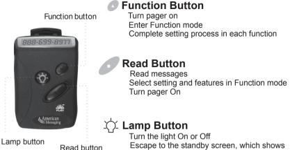
Escape to the standby screen, which shows time, date, alarm status, and alert status. Press  $\Delta^{t}$  twice to escape to the standby screen
